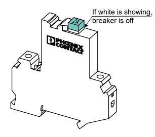
After all your connections have been made, locate this breaker switch in the AE Panel and make sure the breaker button is depressed. Tip: If the white ring is showing on the button, the button is not fully depressed.
