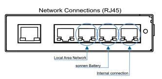
Locate the ethernet switch that is mounted under the DIN-RAIL (lower right of the panel).
