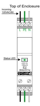
\*Connect high voltage cable to the PLUGTRAB. (Located in the upper left of the panel)
