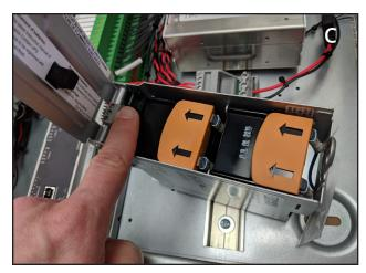
Once the UPS battery case is open, locate the fuse holder, towards the bottom left of the battery enclosure, and insert the fuse.
